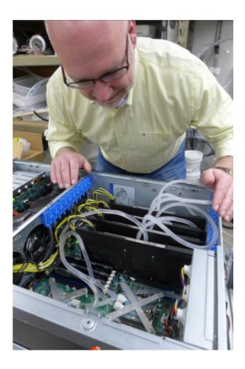
Timothy Shedd examines a computer equipped with his novel cooling system. Tubes circulate refrigerating fluid through a special heat exchanger (under the X-shaped structure) on the processor that is the biggest heat source in a computer. Credit: David Tenenbaum
