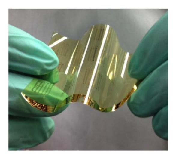
Stanford engineers have developed an improved process for making flexible circuits that use carbon nanotube transistors, a development that paves the way for a new generation of bendable electronic devices. Credit: Bao Lab, Stanford University
