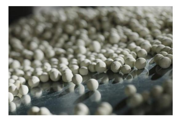
Zeolites are crystalline minerals with a porous structure that adsorbs other substances. When the material comes into contact with water vapor, it binds the steam within its pores, releasing heat in the process. Credit: © Fraunhofer IGB
