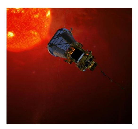
Artist's impression of NASA's Solar Probe Plus spacecraft on approach to the sun. Set to launch in 2018, Solar Probe Plus will orbit the sun 24 times, closing in with the help of seven Venus flybys. The spacecraft will carry 10 science instruments specifically designed to solve two key puzzles of solar physics: why the sun's outer atmosphere is so much hotter than the sun's visible surface, and what accelerates the solar wind that affects Earth and our solar system. The
