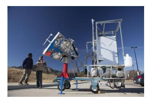
CU-Boulder postdoctoral researcher Tesfayohanes Yakob, left, and research engineer Dana Haushulz are shown here with a novel solar-thermal toilet developed by a team led by CU-Boulder Professor Karl Linden as part of the Bill & Melinda Gates Foundation's "Reinvent the Toilet Challenge" to improve sanitation and hygiene in developing countries. Credit: University of Colorado
