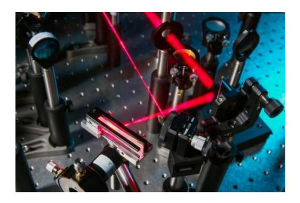
Lasers and complex optic techniques are used to observe molecular interactions at water/oil interface.
