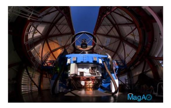
The Magellan Telescope with the MagAO's Adaptive Secondary Mirror mounted at the top looking down some 30 feet onto the 21-foot diameter primary mirror, which is encased inside the blue mirror cell. Credit: Yuri Beletsky, Las Campanas Observatory
