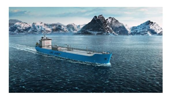
LNG carriers transport liquefied natural gas at very low temperatures to compress gas volumes. Depicted here is a small-scale LNG carrier featuring prismatic tanks designed and developed by LNG New Technologies. (Illustration: LNG New Technologies AS / Michael Grebstad)
