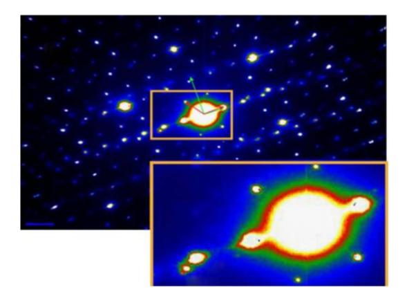
This nano-beam electron diffraction pattern of rhenium disulfide with a zoom-in insert image reveals a quasi-hexagonal reflection pattern. Credit: Junqiao Wu, Berkeley Lab
