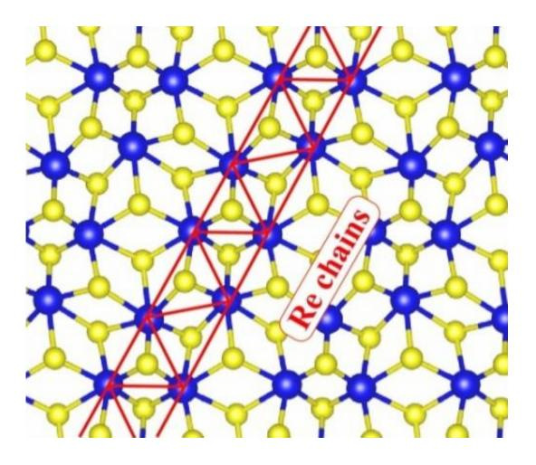
The atomic structure of a monolayer of rhenium disulphide shows the dimerization of the rhenium atoms as a result of the Peierls, forming a rhenium chain denoted by the red zigzag line. Credit: Junqiao Wu, Berkeley Lab
