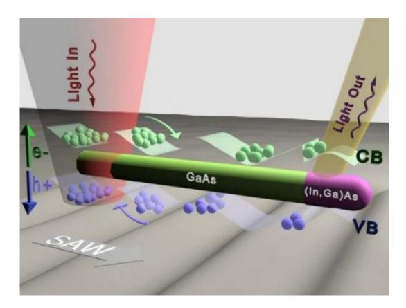
The technology developed at MESA+ and the PDI allows that this can be all done at very high frequencies (over 1 GHz) and at the nanoscale. This opens up the way for applying this kind of devices for quantum information processing as well.
