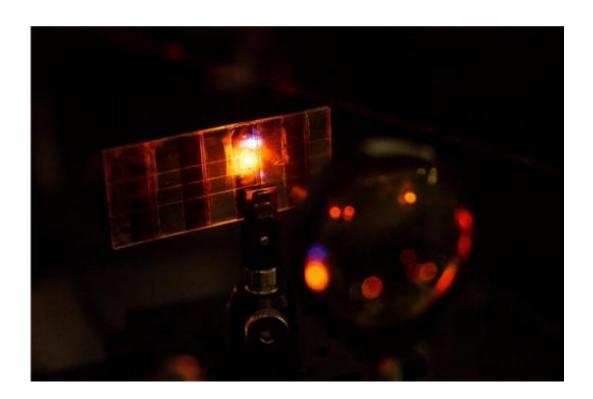
NTU's new Perovskite solar cell as seen in the lab, which was found have light emitting properties.
