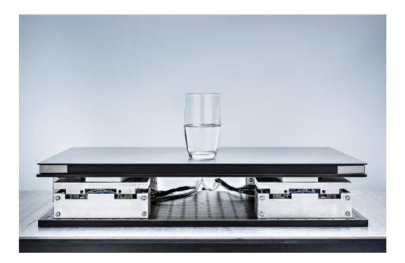
Platform dampens vibrations in all spatial directions. Credit: Fraunhofer LBF
