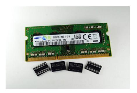
In addition, the new 20nm 4Gb DDR3- based modules can save up to 25 percent of the energy consumed by equivalent modules fabricated using the previous 25 nanometer process technology. This improvement provides the basis for delivering the industry's most advanced green IT solutions to global companies.
