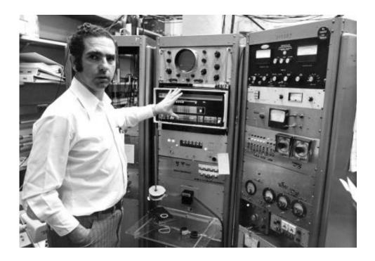
A 1974 photo of Aron Kuppermann standing in his lab with a piece of equipment called a molecular beam machine—used to study the same reaction that was being calculated on the computer at ambassador college. The machine included several pieces of electronic equipment that were controlled by a minicomputer. Credit: Caltech Archives
