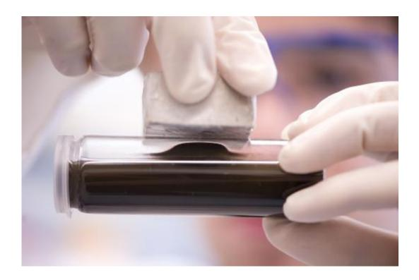
Using magnets the superparamagnetic particles in the water can be removed along with their phosphorus load. Credit: Knut Dobberke / Fraunhofer ISC
