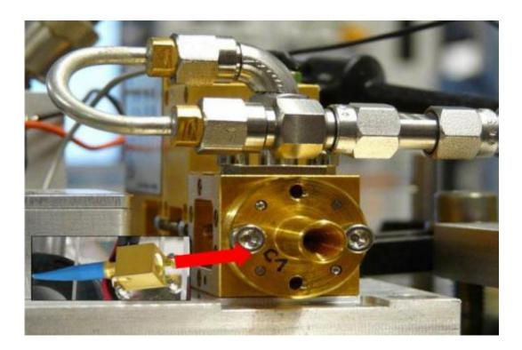
The transmitter (inset) and the receiver of the system.
