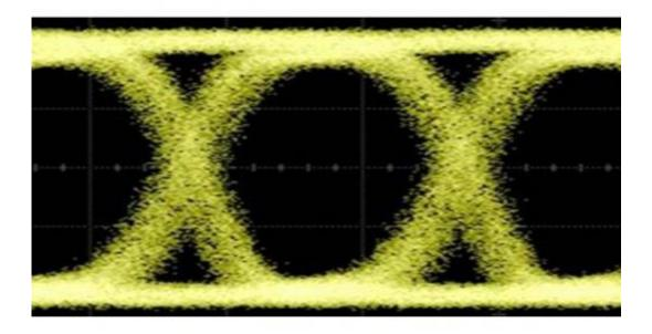
An eye diagram of a 10 Gbit/s signal sent and received using the system.
