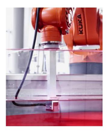
The probe generates ultrasonic waves that penetrate the ma-terial. Credit: Uwe Bellhäuser
