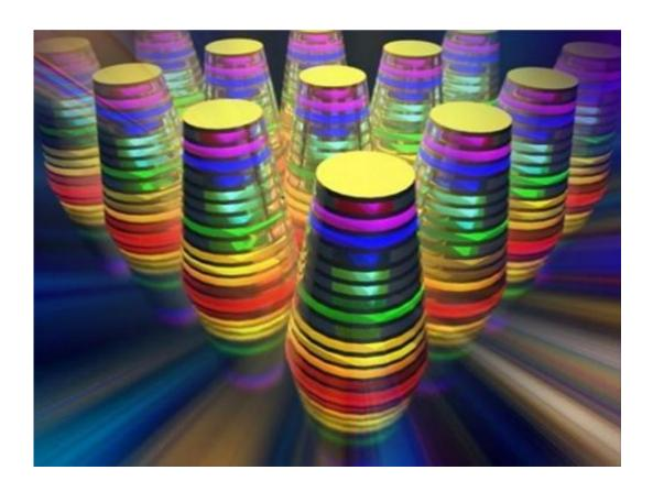
The image shows a 'multilayered waveguide taper array.' The different wavelengths, or colors, are absorbed by the waveguide tapers (thimble-shaped structures) that together form an array. Credit: Qiaoqiang Gan, University at Buffalo
