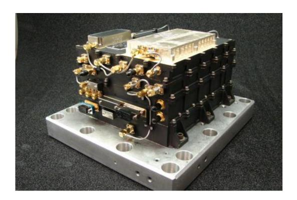
This radio hardware, the Electra UHF Transceiver on NASA's MAVEN mission to Mars, is designed to provide communication relay support for robots on the surface of Mars.
