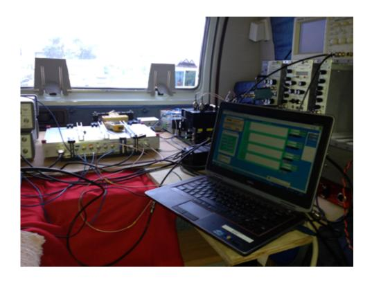
The initial version of the portable frequency comb (inside metal enclosure, left center) is tested as it rides across bumps and dips in the back of a camper van, powered by an on-board generator.
