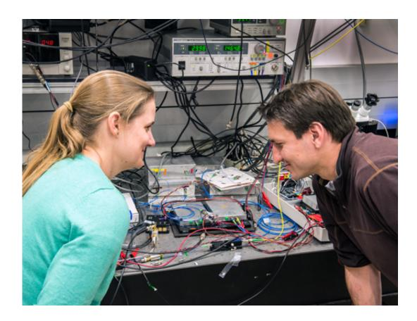
Co-developers Laura Sinclair (left) and Ian Coddington with a test version of the newly miniaturized portable frequency comb that fits in two small metal cases for a total volume of about 1 liter.
