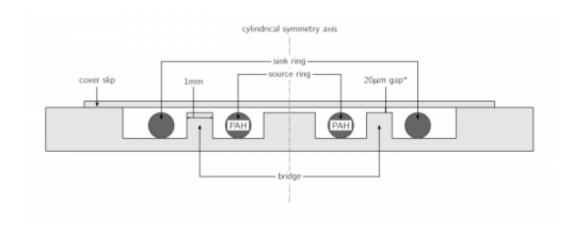
This is a cross-section of a so-called Dunn chamber with two silicone rings. The inner ring contained high concentrations of PAH, whereas the outer ring did not contain any PAH. During the experiments, the ciliates moved from the inner ring, where they absorbed the PAH, to the outer ring, where they released them. Dorothea Gilbert demonstrated this by measuring the content of PAH in the two silicone rings. (\*Gap height 10 times enlarged) Credit: Dorothea Gilbert
