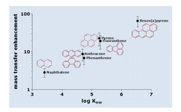
The ciliates' increase of the mobility of PAH grows the more hydrophobic the PAHs are (from the left to the right on the figure) since more PAH is incorporated into the ciliates' fatty cell membrane.  $K_{ow}$  is an expression of chemical compound water solubility. The higher  $K_{ow}$  (octanol:water distribution), the more hydrophobic the PAH (and thereby fat-soluble, lipophilic) are. Credit: Dorothea Gilbert, Aarhus University
