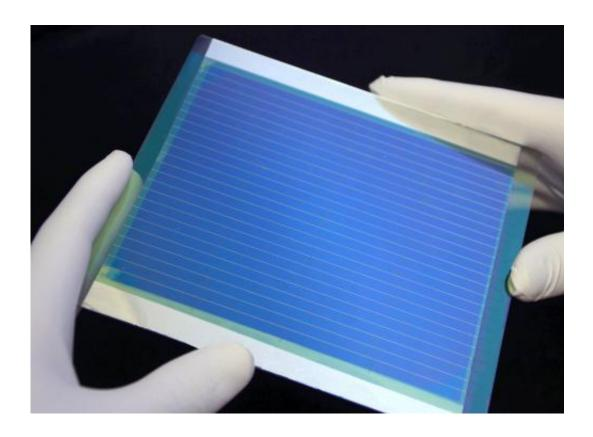
Imec's novel fullerene-free OPV cell concept was used to process an OPV module (156cm2) with a conversion efficiency of 5.3%.
