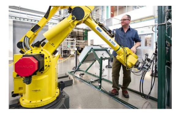
Preparing for the day when hydrogen fueling stations may be as common as gas stations, NREL research engineer Kevin Harrison uses a robot to simulate hydrogen refueling. The robot can simulate the refueling of a vehicle hundreds of times a day. Credit: Dennis Schroeder, NREL
