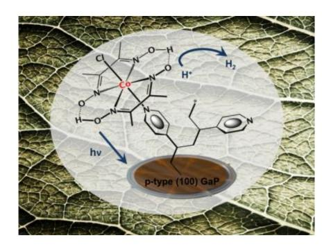
Interfacing the semiconductor gallium phosphide with a cobaloxime catalyst provides an inexpensive photocathode for bionic leaves that produce energy-dense fuels from nothing more than sunlight, water and carbon dioxide. Credit: Gary Moore, Berkeley Lab
