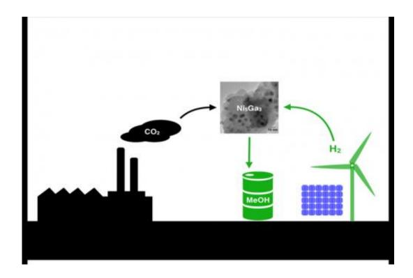
Scientists have created a new nickel-gallium (Ni5Ga3) catalyst that synthesizes methanol (MeOH), a key ingredient in paints and plastics, using carbon dioxide (CO2) and hydrogen (H2). The goal is to create clean methane using hydrogen produced by wind or solar power and CO2 emissions from power plants. Credit: Jens Hummelshoj/SLAC
