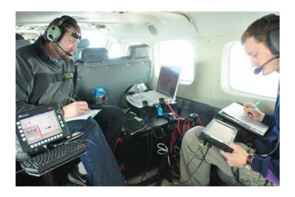
In this photo taken in October 2012, released by WSI, a Quantum Spatial Company, sensor operators Lennie Rummel left, and Drew Wendeborn, right, are shown inside a helicopter taking measurements with LIDAR, a high-tech laser system mounted on the aircraft, to build a detailed elevation map of the terrain above Omak, Wash. The maps can be used by planners and homeowners to begin to assess landslide risk. (AP Photo/ WSI, a Quantum Spatial Company)
