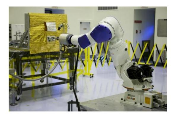
Located at NASA's Kennedy Space Center in Florida, but commanded from NASA's Goddard Space Flight Center in Greenbelt, Md., the RROxiTT industrial robot mimicked how future space robots could transfer oxidizer to a satellite valve. Credit: NASA
