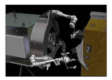
A robot servicer could use autonomous rendezvous and fluid transfer technologies to extend the life of orbiting satellites (depicted, artist's concept). Credit: NASA
