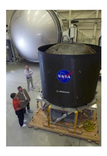
As of 2014, NASA and Boeing are developing a propellant tank made of composite materials to hold cryogenic (low-temperature) gases in space. Initially slated for a 2018 test flight, NASA's 2015 budget will keep these tanks on the ground for the foreseeable future. Credit: NASA/MSFC/Emmett Given
