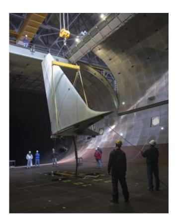
A 40-ton crane carefully lowers the aircraft tail from the rafters down through the open doors of the tunnel's roof. Credit: NASA / Eric James
