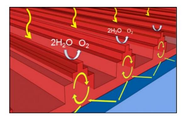
Illustration of a hematite photoelectrode consisting of a periodic nanobeam-array (red) on a conductive ITO layer (dark blue). The nanobeam structure boosts the absorption of sunlight at the hematite/H2O interface, resulting in more efficient conversion of sunlight into solar fuel. Credit: Soo Jin Kim, et al. ©2014 American Chemical Society
