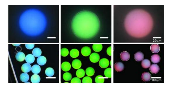
These photonic microcapsules have been prepared to produce blue, green, and red structural colors and imaged using bright-field (top) and dark-field (bottom) optical microscopy. Credit: Jin-Gyu Park, Harvard School of Engineering and Applied Sciences.
