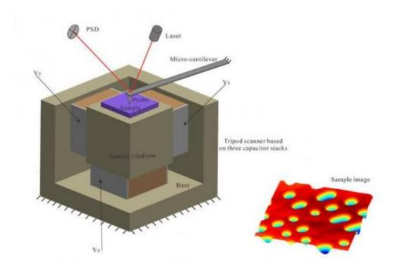
Diagram of a tripod scanning stage based on three X7R MLCCs for an atomic force microscopy AFM imaging system
