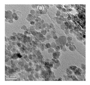
View of unconfined, uncoated iron-oxide nanoparticles as seen via a transmission electron microscope. These nanoparticles, when heated, can be applied to cancer cells in order to kill those cells.
