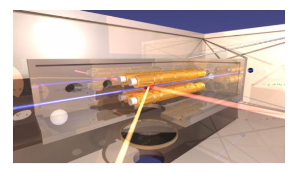
Frozen in the trap: In the Paul trap, which consists of four electrodes, cold helium ions stream in from back left. Collisions with particles of the ion crystal, which is suspended in the center of the trap, cause the noble gas atoms to slow down the rotation of the molecular ions and thus cool their rotational temperature. Credit: J. R. Crespo/O. O. Versolato/MPI for Nuclear Physics
