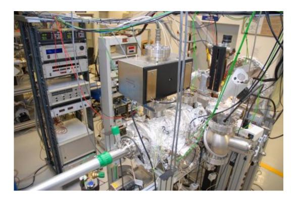
The simulation chamber, named MARTE, is designed to enable study of the behavior of instrumentation and samples of different types and sizes in pressure ranges up to 10-6 mbar controlling the gas composition, with temperature control of samples in the range of 108K to 423K. Credit: J. Martín-Gago/ICMM
