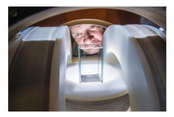
Sandia National Laboratories researcher Jim Martin peers between specially built magnets to watch patterns form in a liquid inside a 3-centimeter (1.2-inch) container. He and Sandia doctoral researcher Kyle Solis have discovered how to harness magnetic fields to create vigorous, organized fluid flows in particle suspensions. Credit: Randy Montoya
