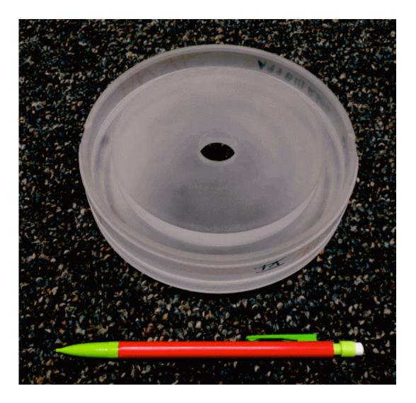
This lithotripsy machine shock wave lens was modified by Duke engineers to more efficiently break up kidney stones. Modifications included a groove cut around the perimeter and an alteration in geometry. Credit: Duke University
