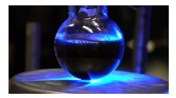
Nano-sized crystals of cobalt oxide, an Earth-abundant catalyst, have been shown to be able to effectively carry out the critical photosynthetic reaction of splitting water molecules. Credit: Roy Kaltschmidt
