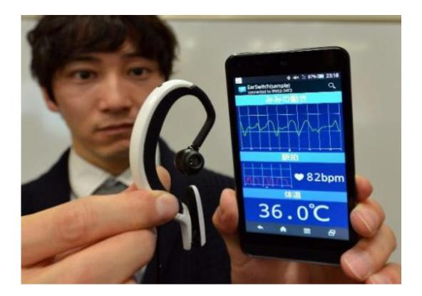
An engineer of Japanese machinery maker NS West shows the 'Earclip-type Wearable PC', equipped with vital sensors, such as pulse meter, thermometer and bluetooth wireless communication device, in Tokyo, on February 20, 2014
