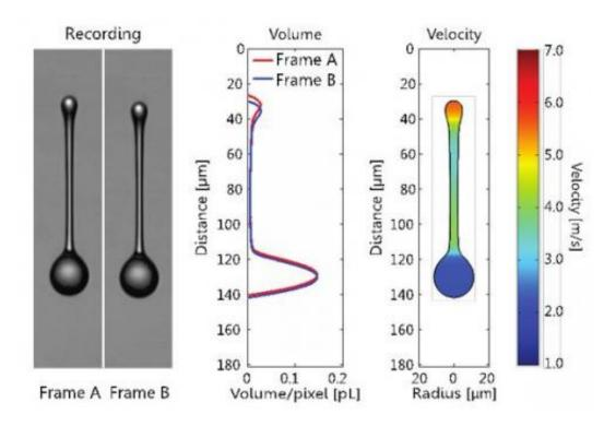
Determining the speed in the microdrops. First a double photo of the same inkjet drop is made, with an interval of 600 nanoseconds. Next the jet and the volume of the drops are determined from the two images. From the movement of the ink in the time between the two photos, the ink speed in the drop can be determined.
