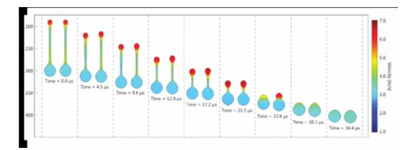
The experimental data (left) are taken as a starting condition for the model (right). The progress of the drop in the model agrees well with the different drops in the experiment at later points in time.
