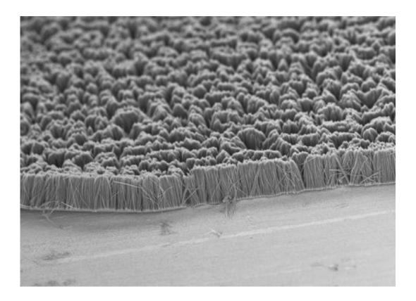
This scanning electron microscope image shows vertical polythiophene nanofiber arrays grown on a metal substrate. The arrays contained either solid fibers or hollow tubes, depending on the diameter of the pores used to grow them. Credit: Virendra Singh
