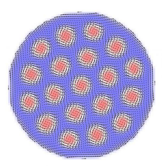
Figure 1: Skyrmions are swirling patterns in the magnetic orientations of atoms (arrows) that can be arranged in ordered patterns. Credit: M. Mochizuki et al.
