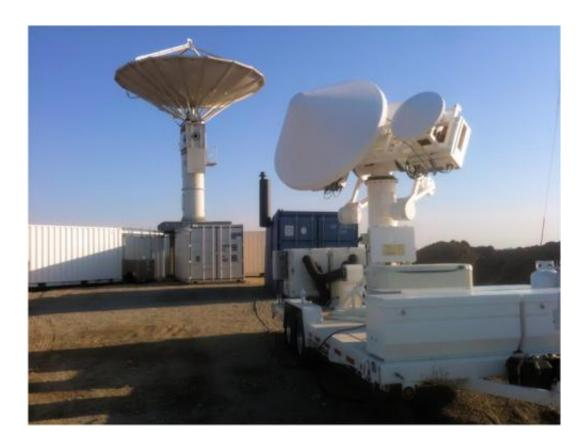
The NASA NPOL (left) and D3R (right) precipitation radars deployed south of Waterloo, Iowa, for the Iowa Flood Studies ground measurement campaign. Credit: NASA/Matt Schwaller
