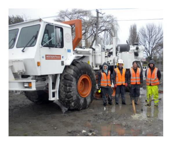
Researchers are using T-Rex, a 64,000-pound shaker truck, in research to increase the resilience of homes and low-rise structures built on top of soils prone to liquefaction during strong earthquakes. T-Rex is based at a University of Texas at Austin facility that is part of the George E. Brown Jr. Network for Earthquake Engineering Simulation (NEES), a distributed laboratory with 14 sites around the United States. Credit: NEES
