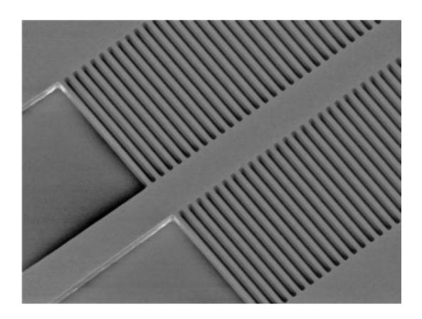
A novel mid-IR waveguide structure for sensing applications.
