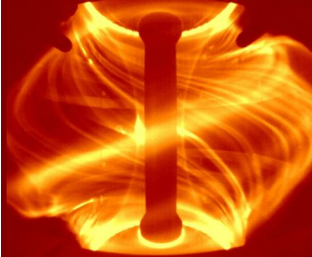
Edge Localized Mode-eruptions in the MAST tokamak, CCFE, UK. Credit: Fundamental Research on Matter (FOM)
