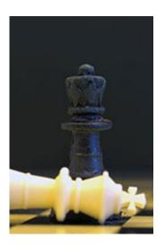
Researchers molded a series of chess pieces made of chitosan bioplastic, demonstrating a new way towards mass-manufacturing large 3D objects with complex shapes made of fully compostable materials. Credit: Harvard's Wyss Institute
