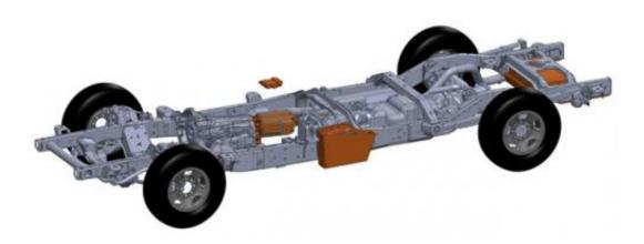
Shown here are XL Hybrids' electric powertrain components (in brown) that attach to traditional gas and oil powertrains. These components include the traction motor (nearest the front), the drive motor (on the side), and the lithium-ion battery (at the rear). Credit: XL Hybrids
