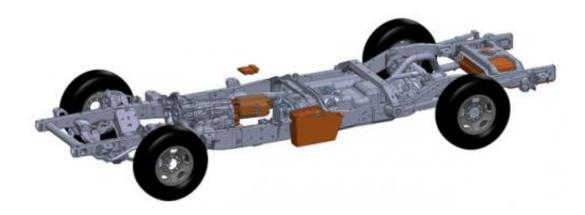
Shown here are XL Hybrids' electric powertrain components (in brown) that attach to traditional gas and oil powertrains. These components include the traction motor (nearest the front), the drive motor (on the side), and the lithiumion battery (at the rear). Credit: XL Hybrids
