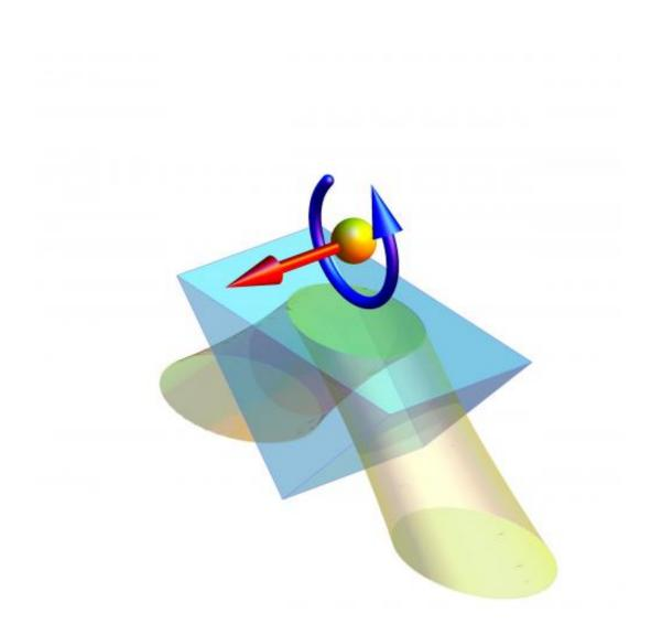
Transverse force and torque on a particle in evanescent field generated from a total internal reflection in a glass prism. These reveal the presence of the transverse momentum and spin in the evanescent wave above the prism. Credit:
