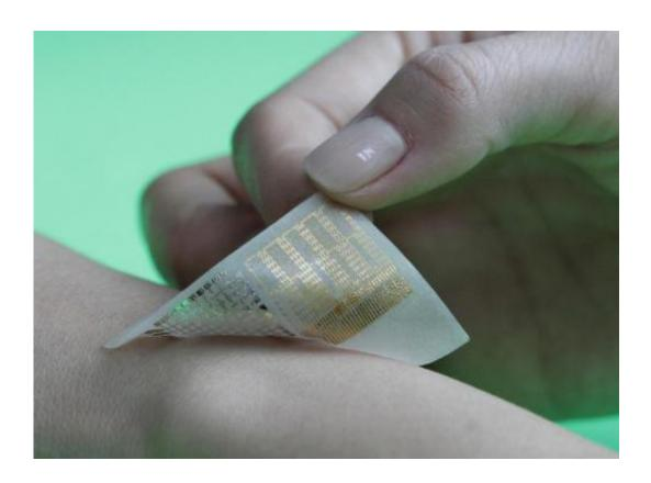
High performance multifunctional wearable electronics integrated with nanoparticles are conformally attached to the skin for the diagnosis and therapy of motion-related neurological disorders. The image shows the multifunctional wearable devices partially peeled away from the skin. Credit: Donghee Son and Jongha Lee
